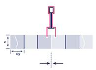
Most Louverlux aluminium louvers can also be installed seamlessly, i.e. the connection between the louver panels is as invisible as possible.
